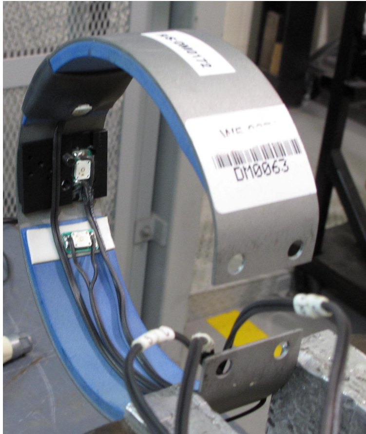
Figure 19. LED cable routing to front of rib
