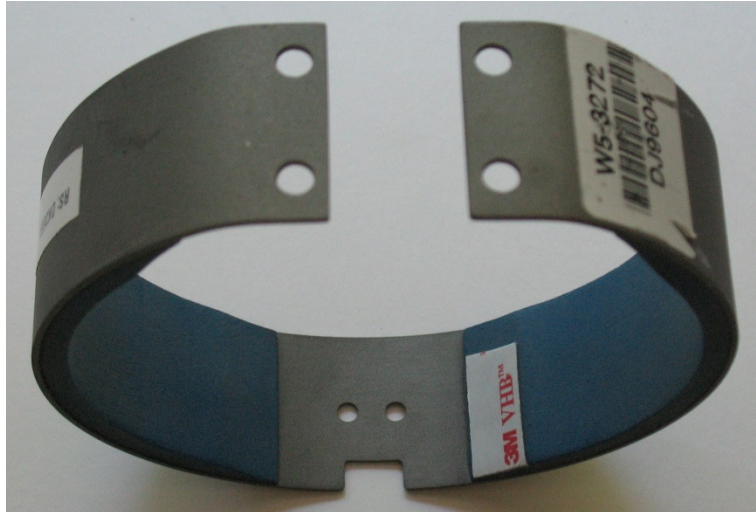
Figure 12. Tape placed at rearward LED location (thoracic 2 rib or abdominal 2 rib shown)
