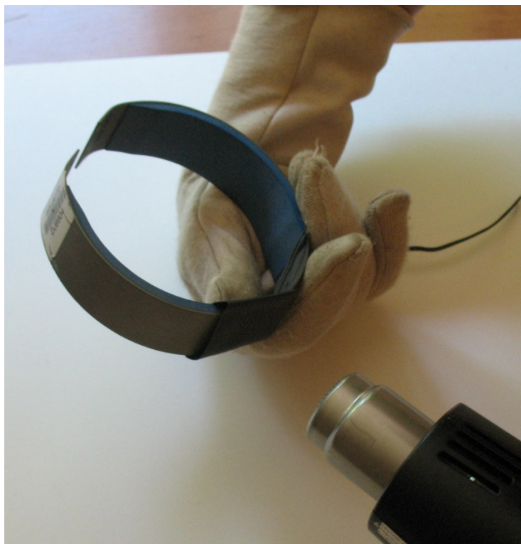
Figure 17. Shrinking outer side of tubing
