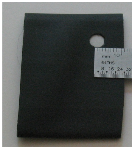
Figure 13. Heat-shrink tubing with hole punched
