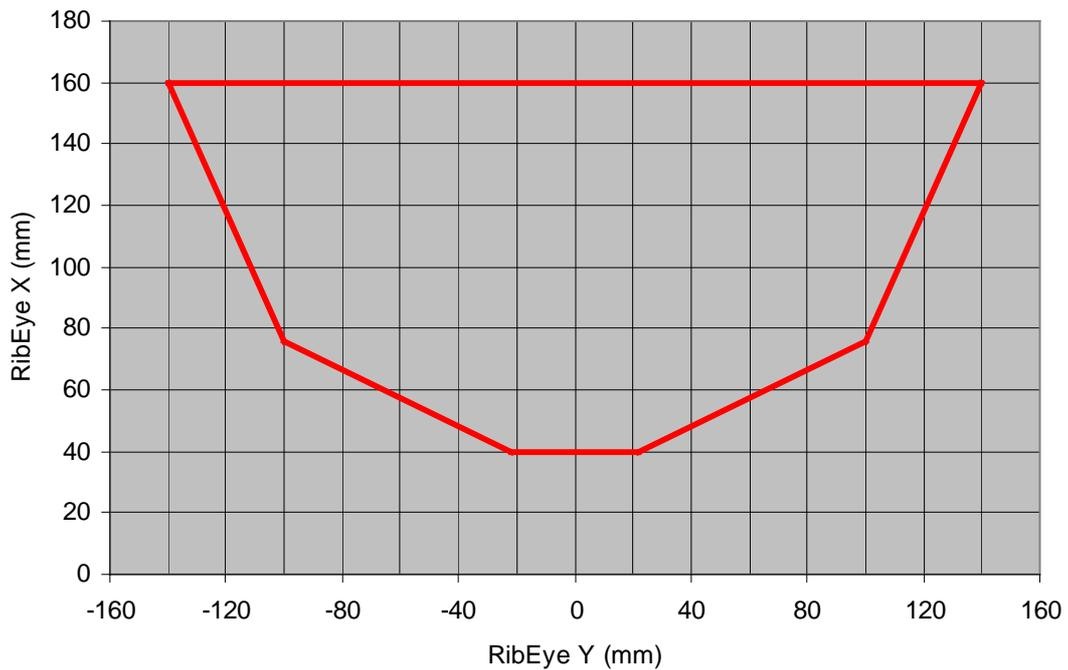
**Figure E1. RibEye measurement range in X-Y plane**
