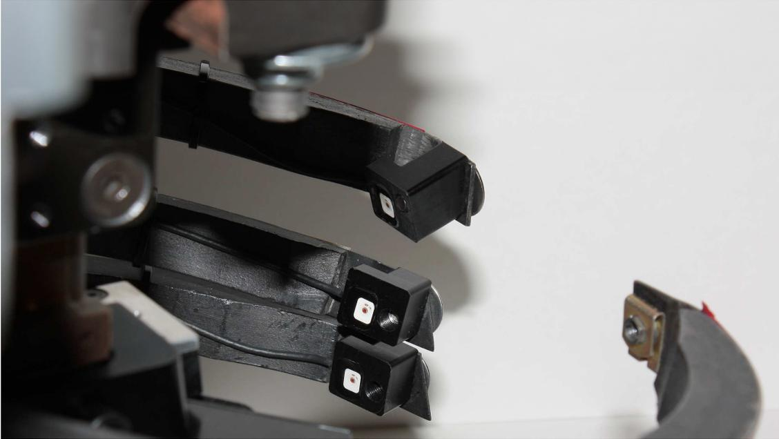
**Figure 7. Mounting LEDs on sternum end of ribs**
