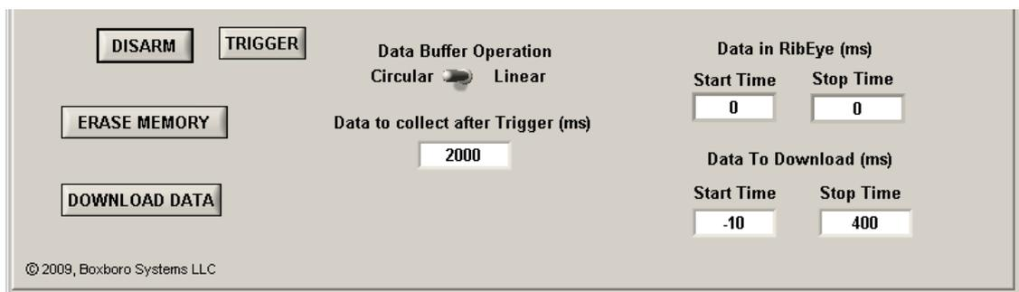
**Figure 15. “Disarm” and “Trigger” buttons that appear after arming**
