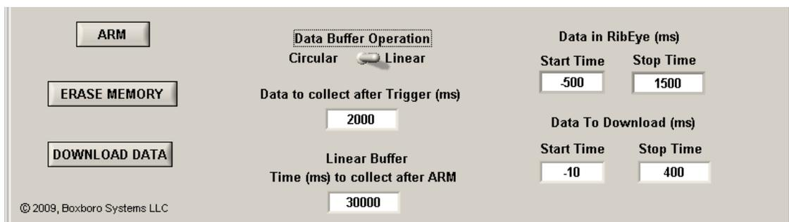
Figure 14. Data collection setup, arm, and download controls
