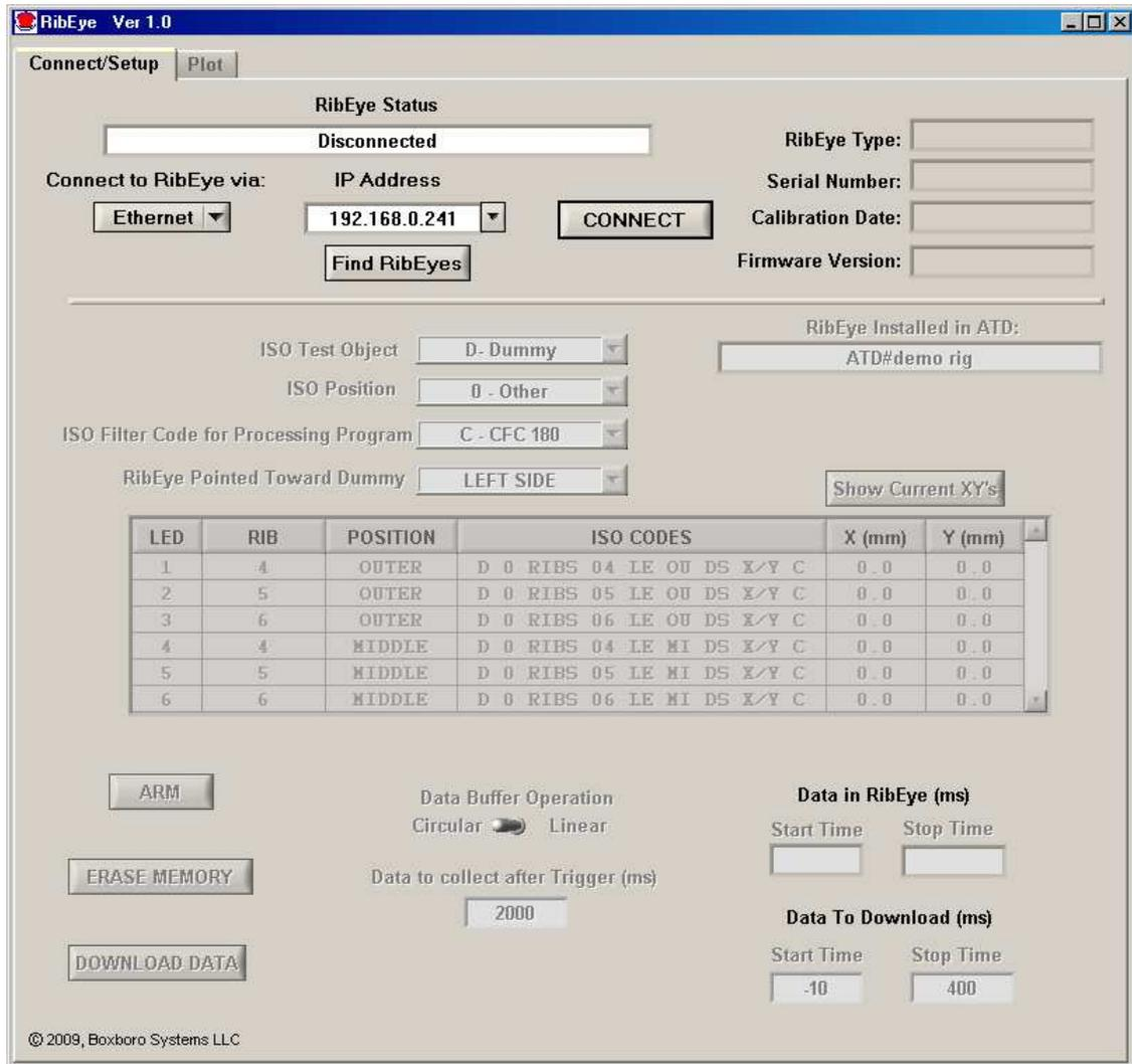
Figure 9. RibEye control software main screen upon start-up
