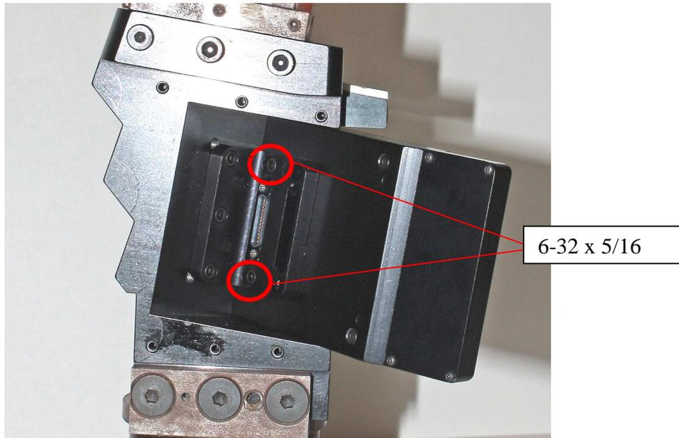
**Figure 5. Mounting RibEye to spine (back side)**
