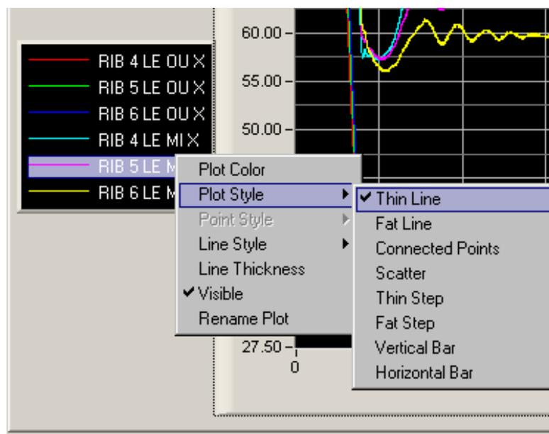
**Figure 18.** Changing plot styles by right-clicking on a trace in the “Legend” box
