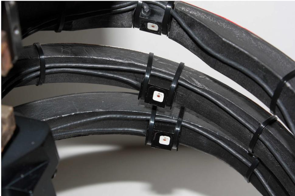
**Figure 6. Mounting outer LEDs on ribs**
