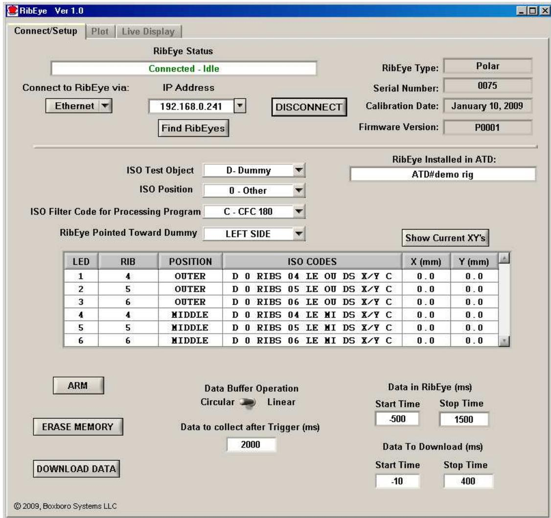
Figure 11. RibEye control software main screen after connecting to RibEye
