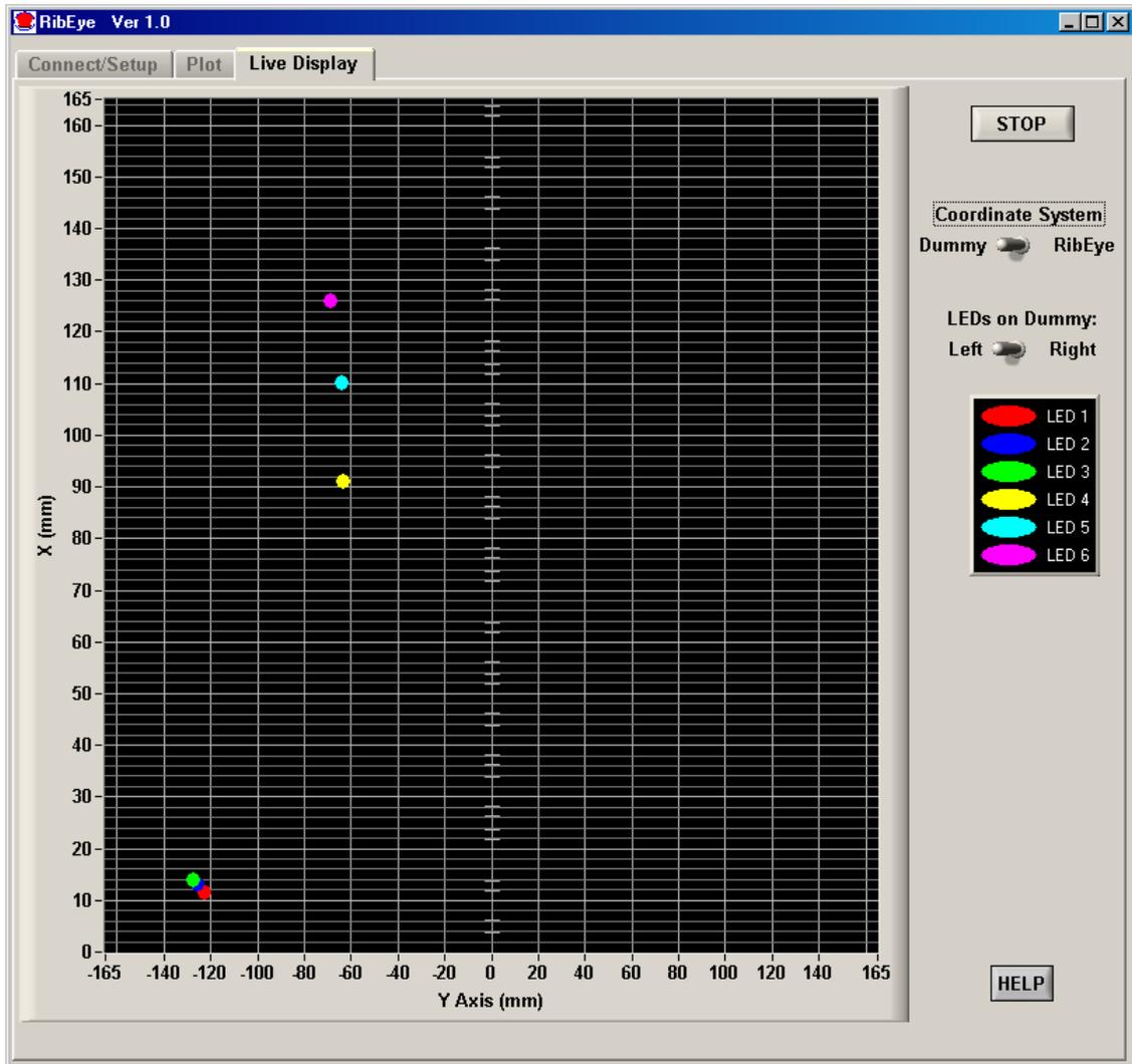
Figure 20. "Live Display" tab with data shown in the dummy coordinate system
