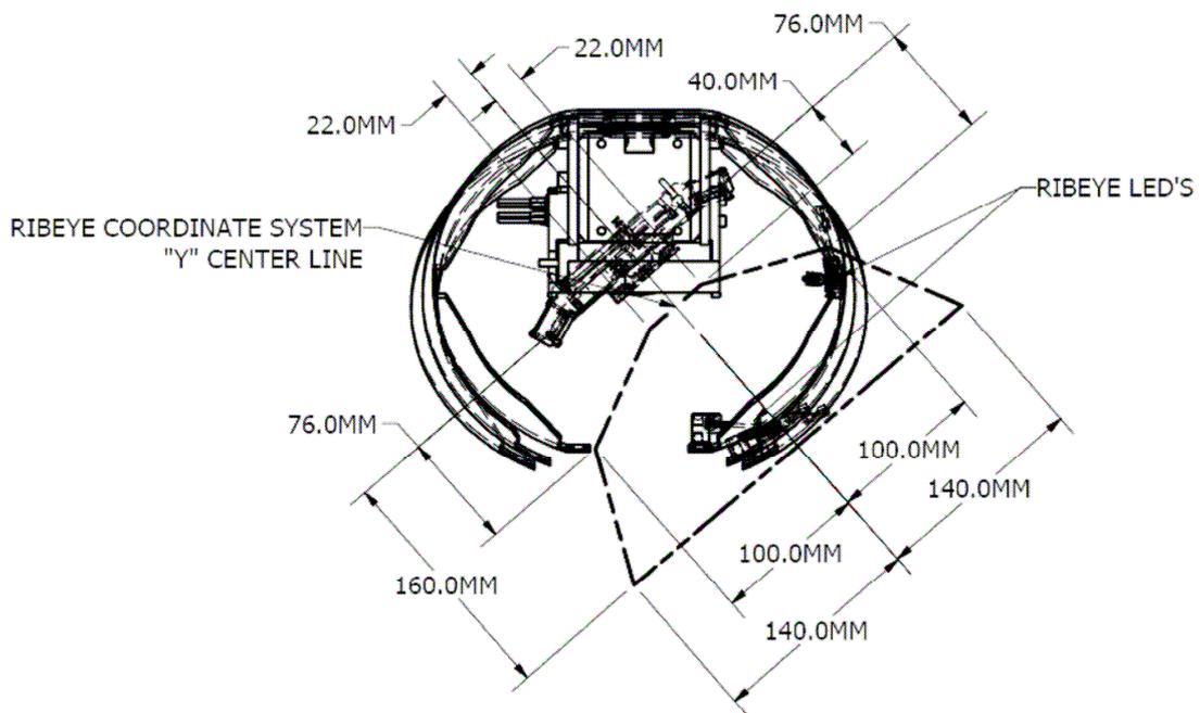
**Figure 3. RibEye measurement range in Polar ATD**
