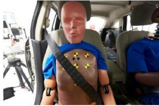
Figure 5. IIHS-conducted Caliber test of small female dummy with forwardmost seat position and D-ring full-down
