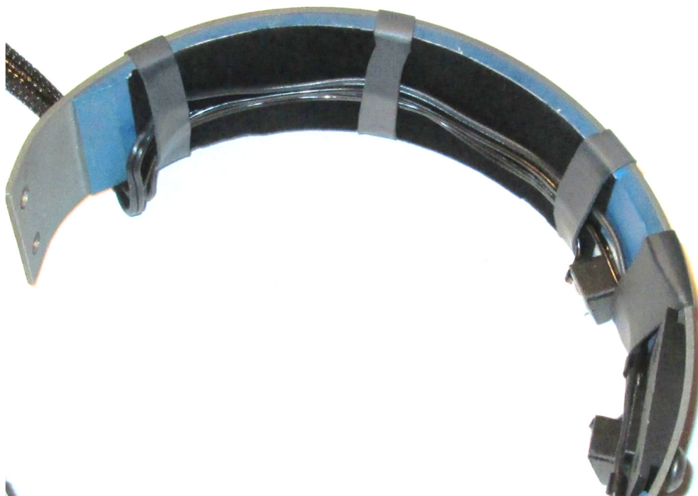
Figure 20. LED cables routed over flock paper
