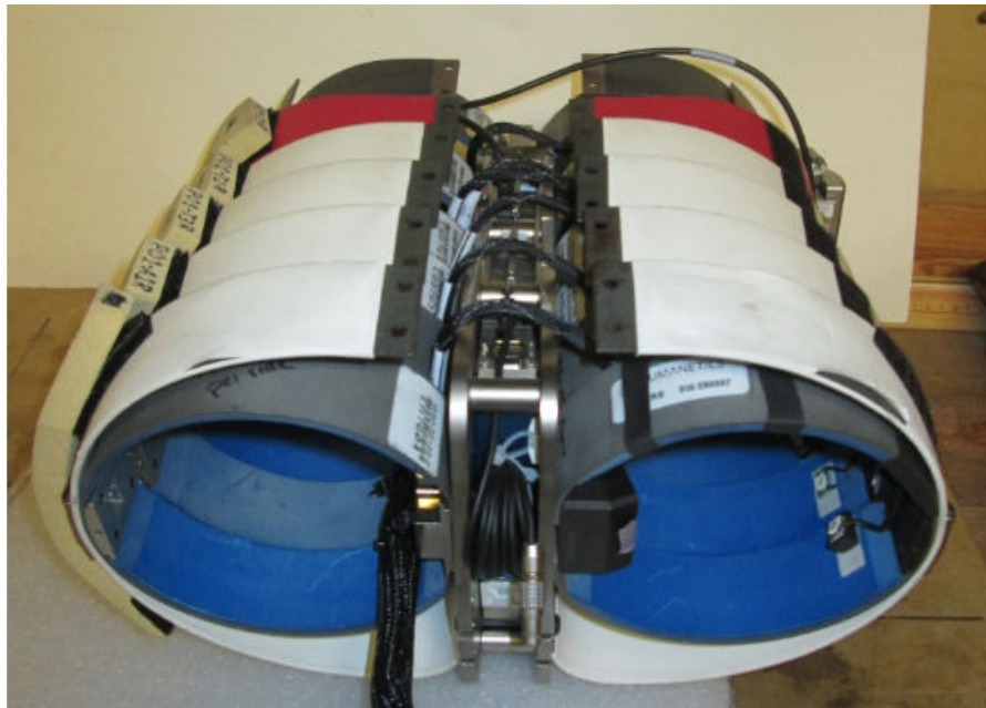
Figure 31. LED routed to non-struck side
